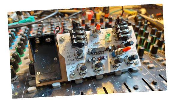
The "LDeRRoR" is a standalone synth devices creating a wide range of square wave noises. It's based on the good old 40106 and it have 6 oscillators, where 3 are duplicated on each output (L+R) and they are mixed via bipolar LED's. So you can send it into a stereochannel for nice droning and panning. Ist controlled via LDR's (light dependend resistors) and with your body (bodycontacts).
